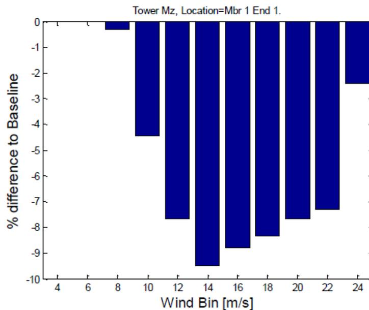
Tower base fatigue load reduction vs wind speed
