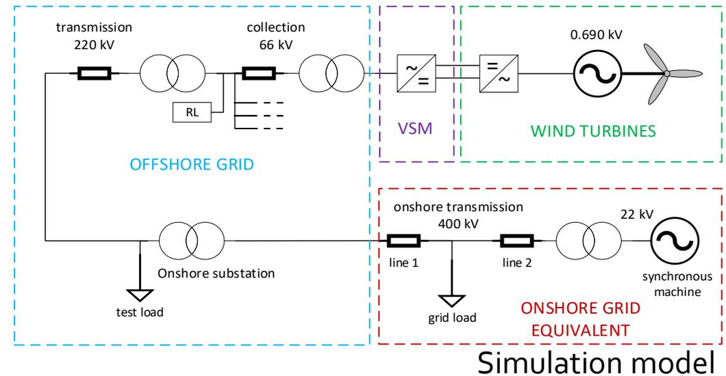
Scheme 1: VSM converter controlling DC voltage - energy drawn only from DC-link capacitor
