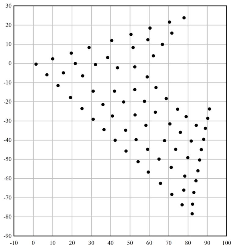
Figure 5: A preliminary layout for the Borssele RWP. This is a semi-regular, perimeter-weighted pattern, and obeys the actual Borssele zone constraints on turbine placement. Axes have units of  $s/D$ , where  $D = 198$  m.
