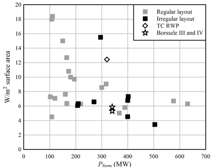
Figure 2: Specific rating (rated power in W / area in m<sup>2</sup>) as a function of rated power for a number of offshore wind power plants. One of the targets of plant control is to make higher specific ratings practical for large plants.
