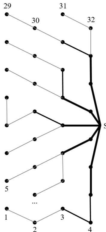
Figure 4: The electrical layout of the TC RWP. Thin gray lines: area 95 mm<sup>2</sup>, ampacity<sup>(1)</sup> 300 A. Thin black lines: 150 mm<sup>2</sup>, 375 A. Thick black lines: 500 mm<sup>2</sup>, 655 A. Turbine identification numbers are shown, and S indicates the location of the electrical substation.
