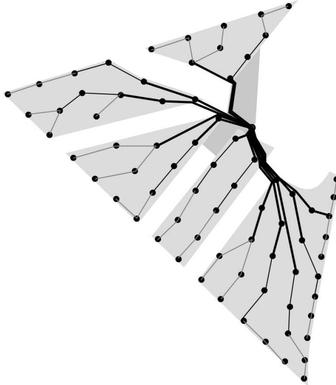
Figure 9: The electrical layout of the Borssele RWP. Thin gray lines: area 95 mm<sup>2</sup>, ampacity 300 A. Thin black lines: 150 mm<sup>2</sup>, 375 A. Thick black lines: 500 mm<sup>2</sup>, 655 A.
