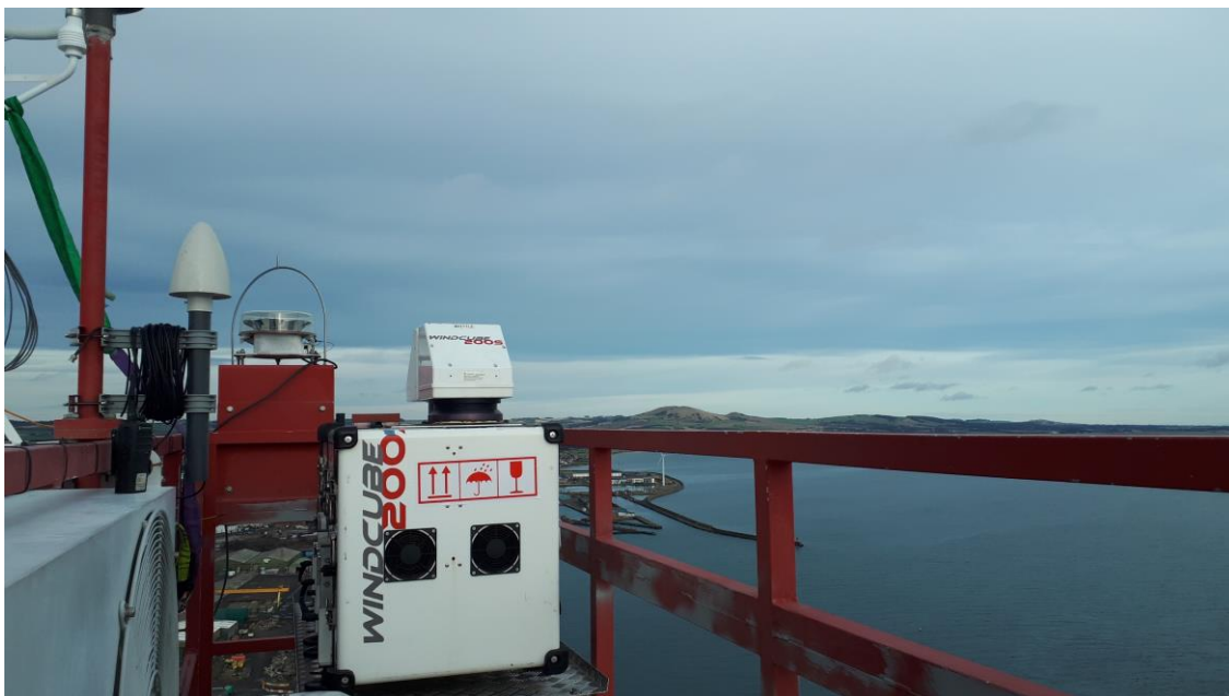
Figure 4 Rear-facing DTU Long-range WindScanner installed on turbine nacelle
