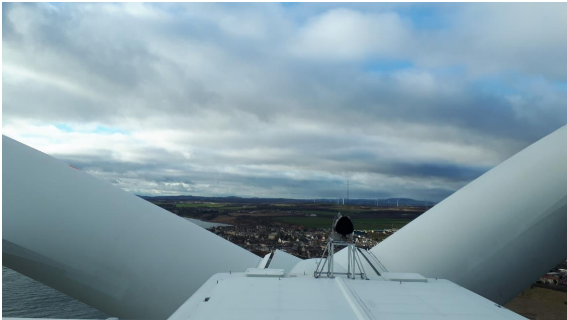
Figure 3 Forward-facing DTU spinner LiDAR installed on turbine nacelle
