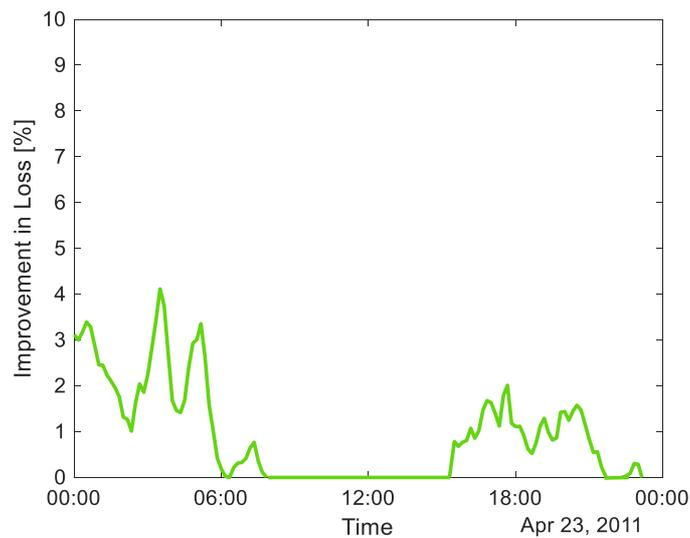
FIGURE 12 IMPROVEMENT IN LOSSES AFTER OPTIMIZATION FOR THE REPRESENTATIVE MEDIUM WIND DAY
