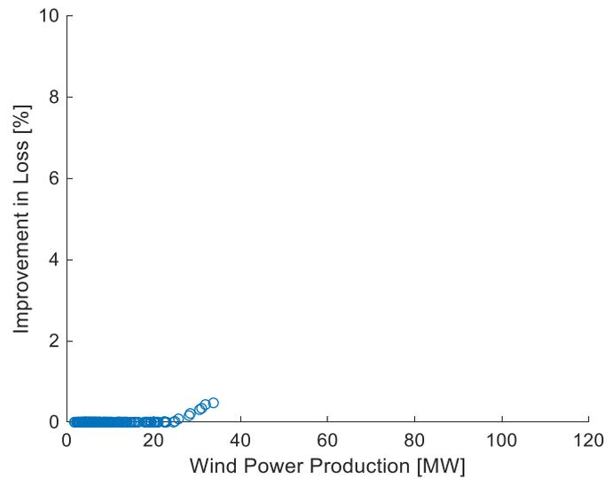
FIGURE 17 IMPROVEMENT IN LOSSES AFTER OPTIMIZATION FOR THE REPRESENTATIVE LOW WIND DAY
