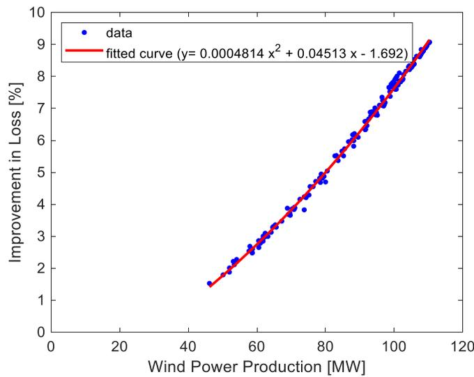
FIGURE 9 CURVE FITTING FOR IMPROVEMENT IN ACTIVE POWER LOSS AGAINST ACTIVE POWER PRODUCTION DURING HIGH WIND SCENARIO
