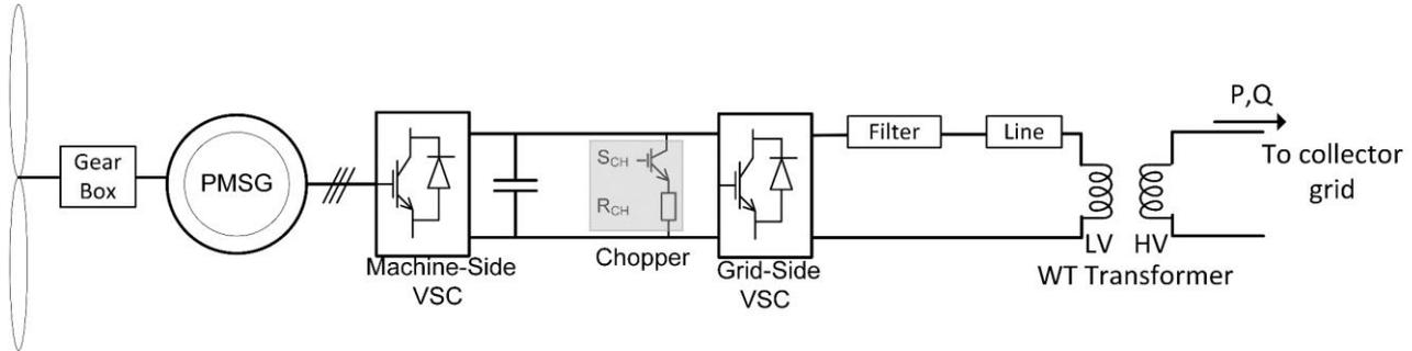
FIGURE 3 SCHEMATIC DIAGRAM OF FULLY RATED CONVERTER BASED WIND TURBINE
