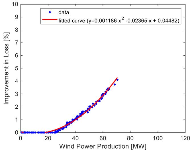
FIGURE 14 CURVE FITTING FOR IMPROVEMENT IN ACTIVE POWER LOSS AGAINST ACTIVE POWER PRODUCTION DURING MEDIUM WIND SCENARIO
