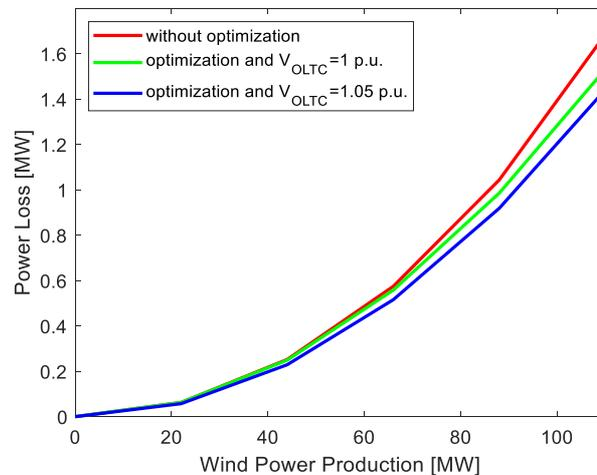
FIGURE 19 ACTIVE POWER LOSS WITHOUT OPTIMIZATION AND WITH OPTIMIZATION FOR DIFFERENT OLTC SETTINGS
