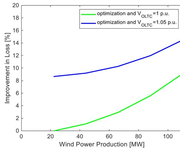
FIGURE 20 IMPROVEMENT OF LOSSES FOR DIFFERENT OLTC SETTINGS
