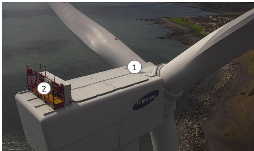
Figure 8 Lidar installation locations - front-facing lidar on nacelle roof (1) and rear-facing lidar on rear gantry (2)
