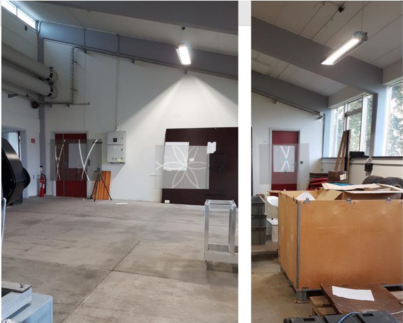
Figure 4 Scan pattern from the spinner lidar recorded on the wall
