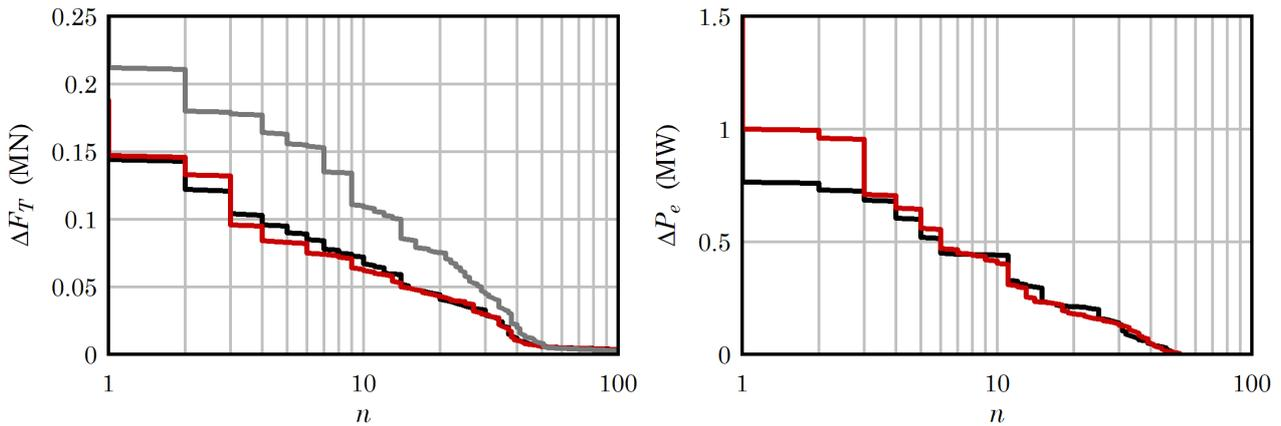
Figure 38: Rainflow-count exceedance curves of thrust and power for Turbine 1. Gray: constant power command (Scenario 1). Black: damage = 0 (Scenario 2). Red: Turbine 1 damage = 1 (Scenario 3). The gray curve is near zero in the right-hand plot. For an example of how to interpret these curves, the gray curve in the left-hand plot indicates that there are about 100 total cycles; 40 cycles that exceed an amplitude of 0.02; 10 cycles that exceed an amplitude of 0.11; and so on.
