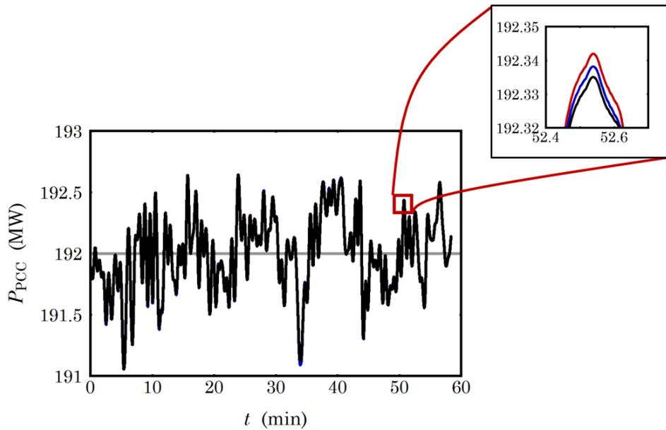
Figure 37: The power at the PCC, where the set-point is 192 MW, or 6 MW per turbine on average. Gray line (flat at 192 MW): constant set-point. Red: zero damage. Blue: Turbine 1 unit damage. Black: random damage.
