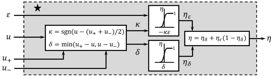
Figure 8: The block providing anti-windup features.
