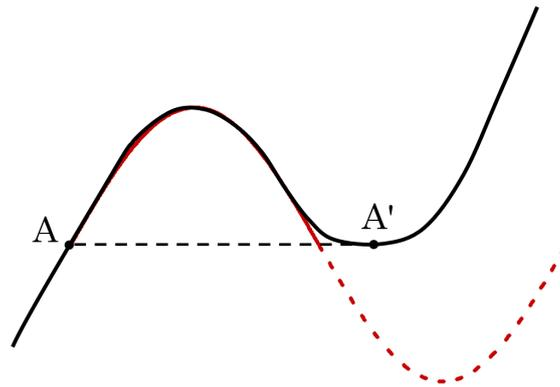
Figure 20: A half rainflow cycle A-A', approximated as part of a sinusoid.
