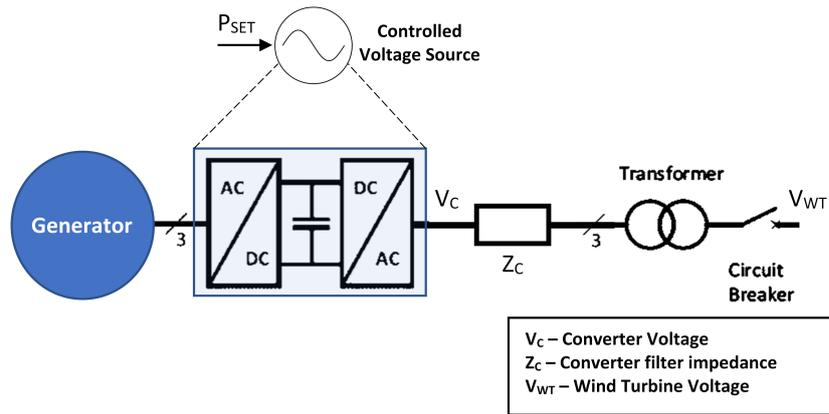
Figure 43: Simplified representation of electrical power train.
