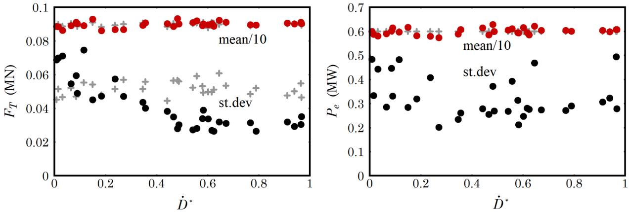
Figure 39: Trends in the mean and standard deviation of thrust and power fluctuations, as a function of damage rate (Scenario 4). Nominal results for the case with a constant power command (Scenario 1) are shown in the background.
