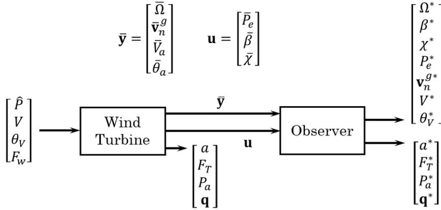
Figure 26: The architecture used to test the observer.
