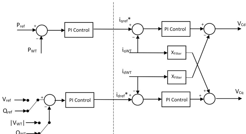
Figure 45: Control loops of Grid Side Converter.
