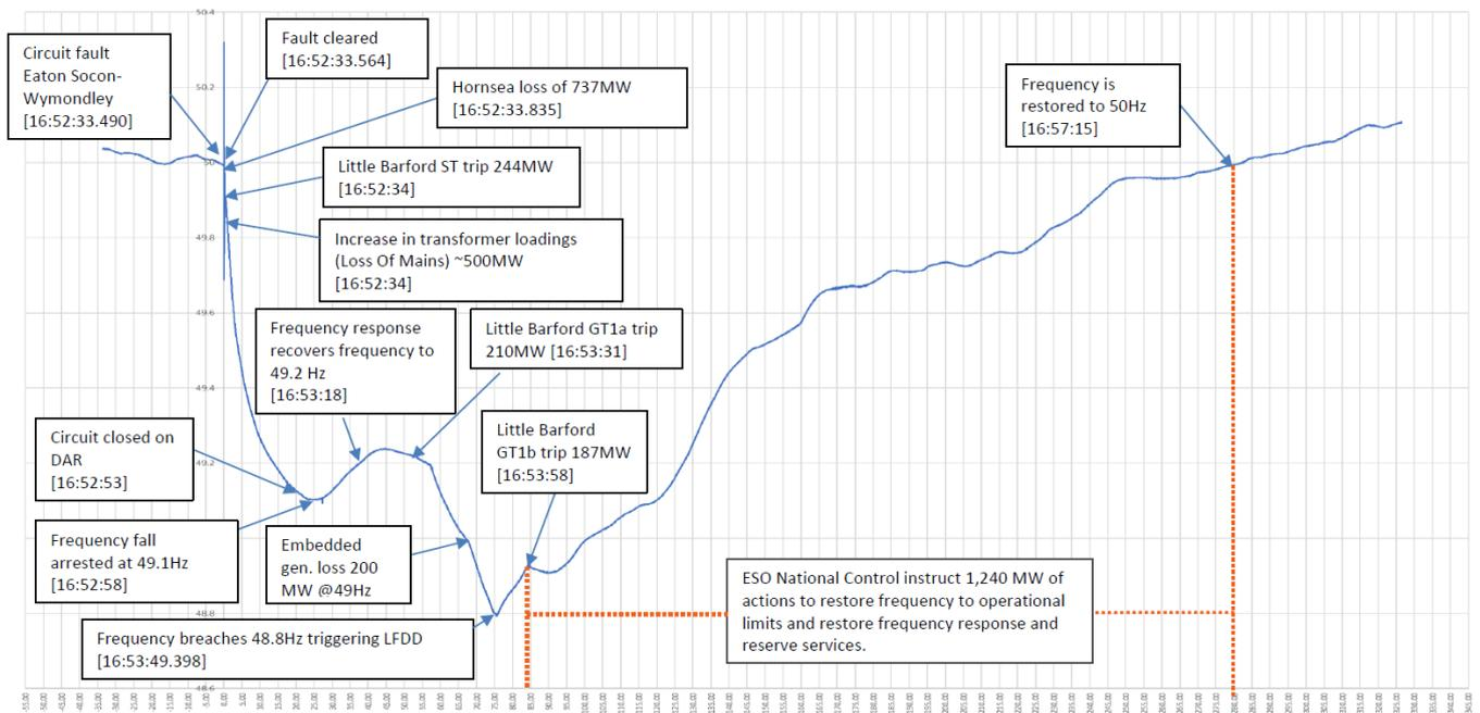
Figure 52: Annotated frequency trace of the partial black-out event in August 2019 (National Grid ESO 2019).
