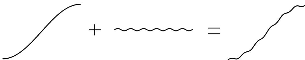
Figure 19: How cycles may be lost when low and high frequency signals are combined.
