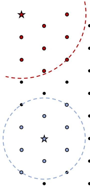
Figure 13: Examples of two turbine clusters, used to estimate the “mean” wind speed and direction at the starred turbines.
