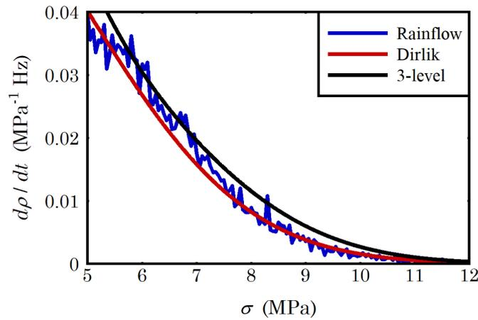
Figure 24: A close-up of the tail of the left-hand plot in Fig. 23, with a linear scale.
