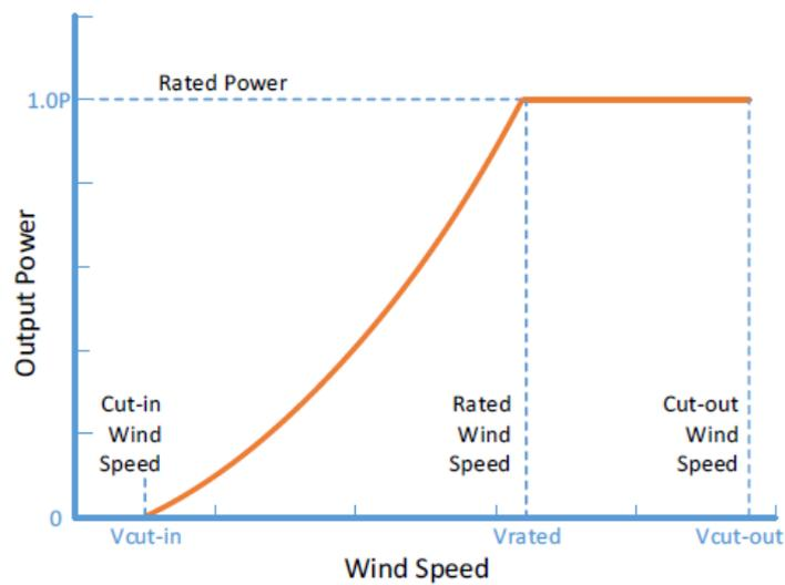
Figure 50: Power curve of a wind turbine.
