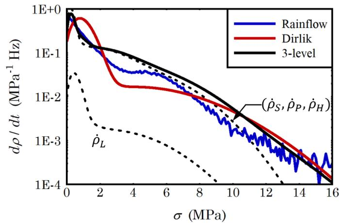
Figure 25: Combined  $(n_L, n_S, n_P, n_H)$  cycles, expressed as density rate curves, for the point dominated by flapwise moments.
