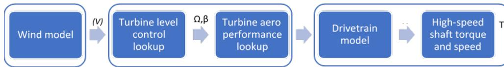
Figure 46: Block diagram of model for aero-mechanical power train.
