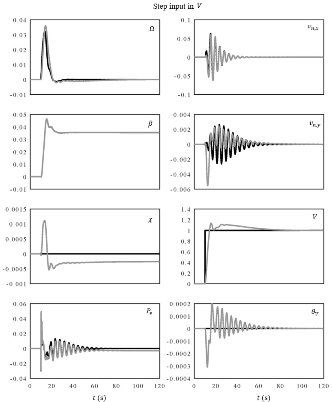
Figure 29: The response of sensor outputs to a unit step change in the wind speed.
