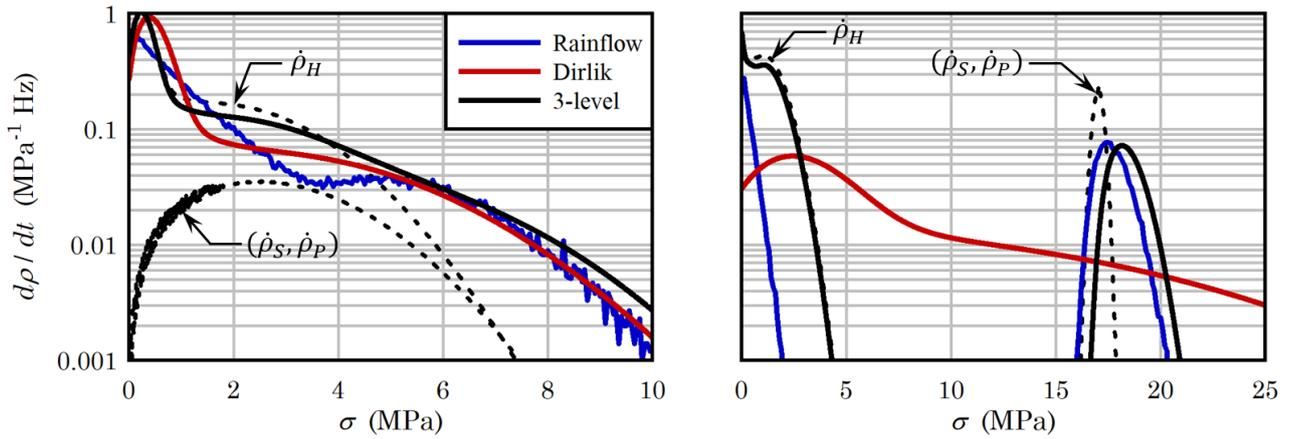
Figure 23: Combined  $(n_S, n_P, n_H)$  cycles, expressed as density rate curves. Counts obtained by the rainflow method are compared with those from Dirlik’s equation and the proposed three-level method. The plot at left shows a point dominated by flapwise moments, while at the right is a point dominated by edgewise moments.
