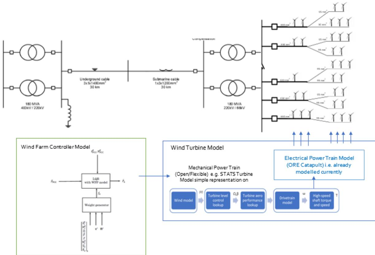
Figure 51: Block diagram of integrated WT/WPP control/PSCAD model.
