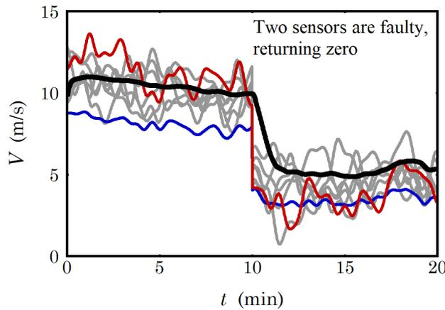
Figure 34: The cluster wind speed estimate with a step input of  $-5$  m/s at  $t = 10$  minutes. Two sensors are faulty and are returning zero; the cluster wind speed (black curve, see Fig. 33 for the legend) is to be compared with plain averaging of the signals (blue curve).
