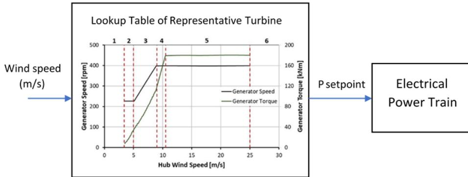
Figure 47: An example of option 2 with lookup tables of wind turbine speed and power curves.
