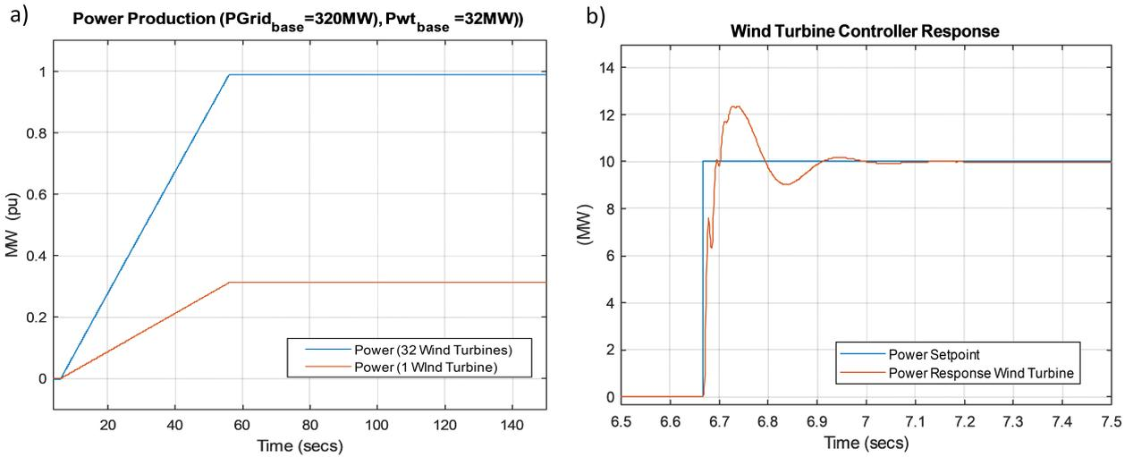
Figure 49: Simulation Results: (a) Power production with the wind turbines, (b) wind turbine controller electrical power response.
