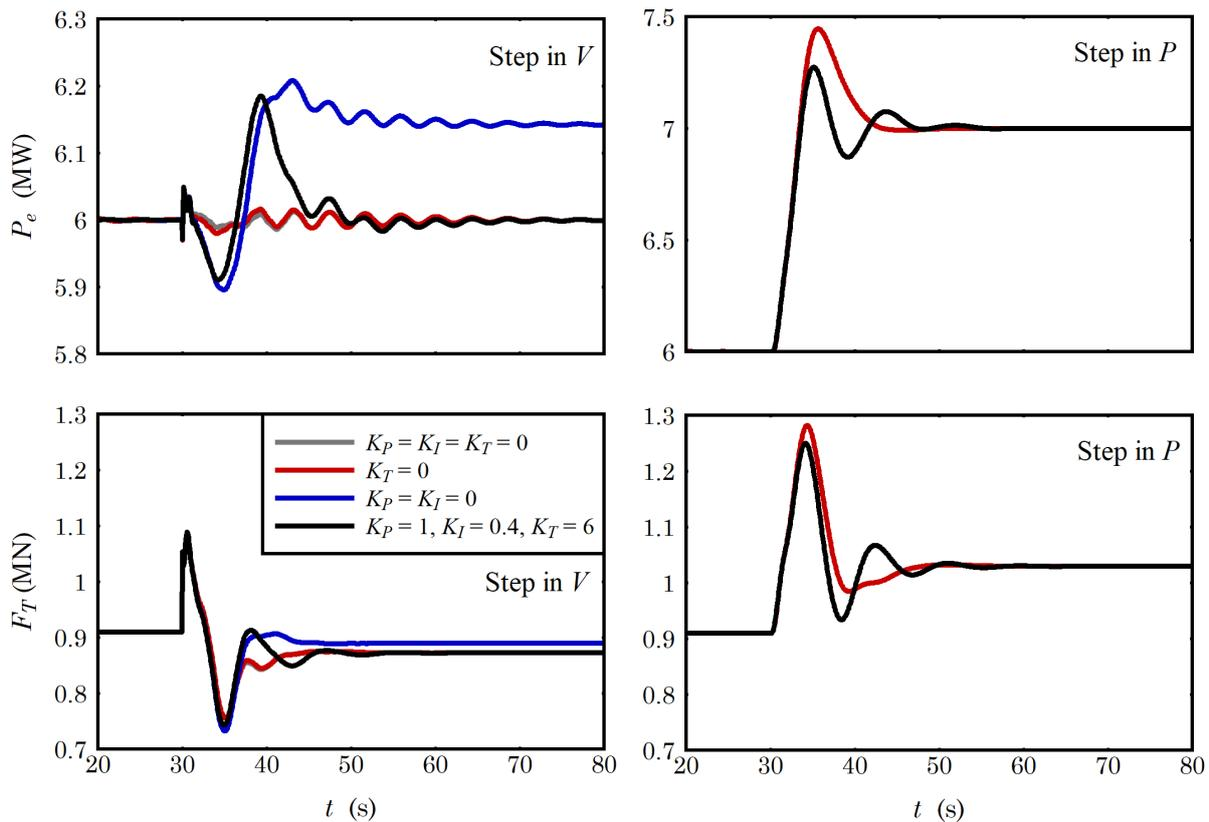
Figure 32: The response of electrical power (at top) and rotor thrust (at bottom) to unit step inputs in wind speed (at left) and power command (at right), with different gains.
