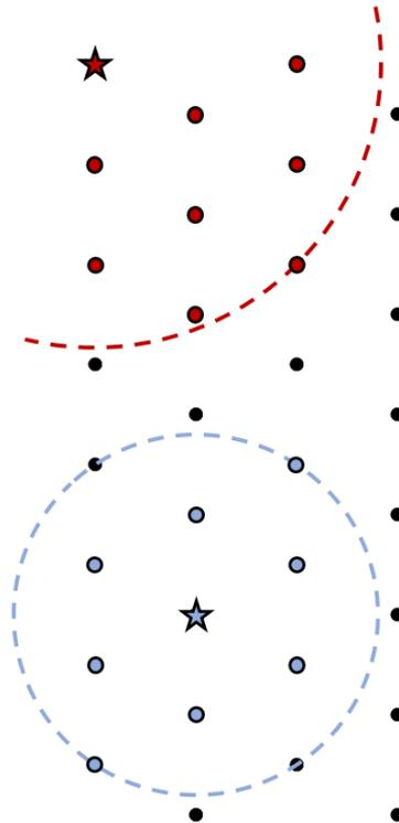
Figure 13: Examples of two turbine clusters, used to estimate the “mean” wind speed and direction at the starred turbines.
