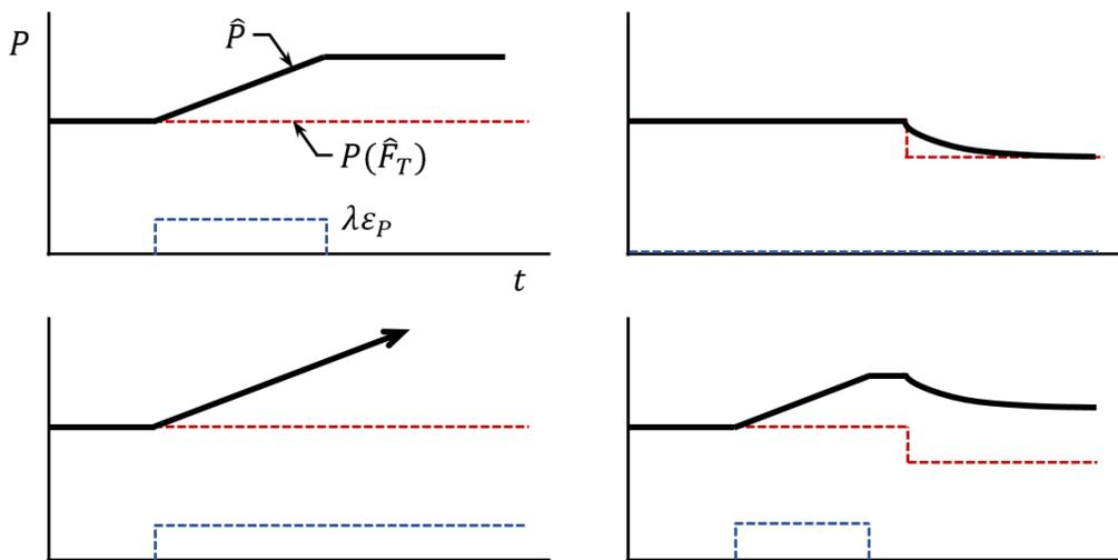
Figure 5: Sketches of the desired response characteristics of the commanded power  $\hat{P}$  under different combinations of power-tracking  $\lambda\epsilon_P$  and thrust-tracking  $P(\hat{F}_T)$  errors.
