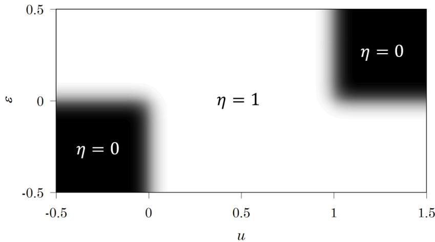
Figure 9: Output of the anti-windup block for a case in which the valid range of  $u$  is between 0 and 1. The smoothed transition between  $\eta = 0$  and  $\eta = 1$  is convenient for numerical solution of the nonlinear state equations.
