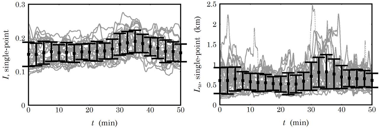
Figure 36: Single-point turbulence intensity and length scale for each turbine, derived from the turbulence cascade after a 10-minute burn-in period. The error bars indicate the standard deviation.
