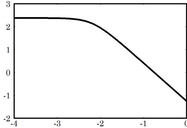
Figure 15: An example of the Von Karman spectrum,  $\mu_V = 10 \text{ m/s}$ ,  $I = 0.183$ ,  $L_u = 180 \text{ m}$ .
