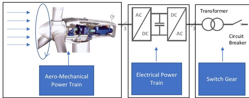
Figure 41: High level description of the Wind Turbine Model in PSCAD.
