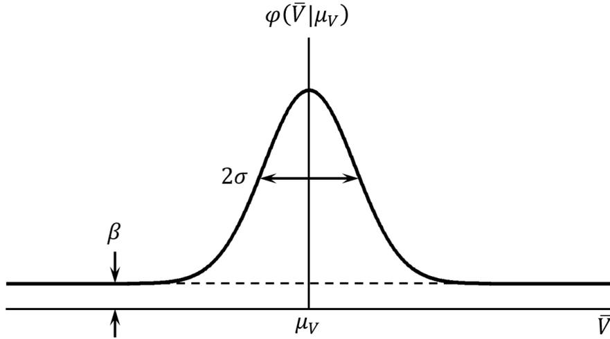
Figure 14: A two-parameter distribution representing the uncertainty in measurements at a single turbine, given a value of the cluster average.
