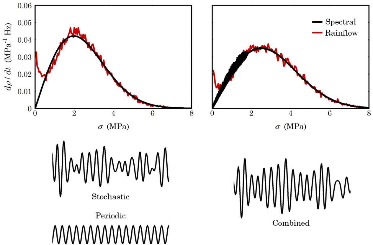
Figure 17: Cycle count density rate curves from the stochastic and periodic blade root stress spectra near the 1P frequency, along with samples of the corresponding time series. Stresses at this location are dominated by flapwise bending.
