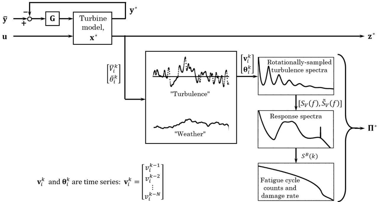
Figure 10: The architecture of the state observer, showing the embedded wind turbine model, a module that distinguishes local turbulence from broader weather patterns, and an analytical spectral model that estimates the severity of loading and fatigue.
