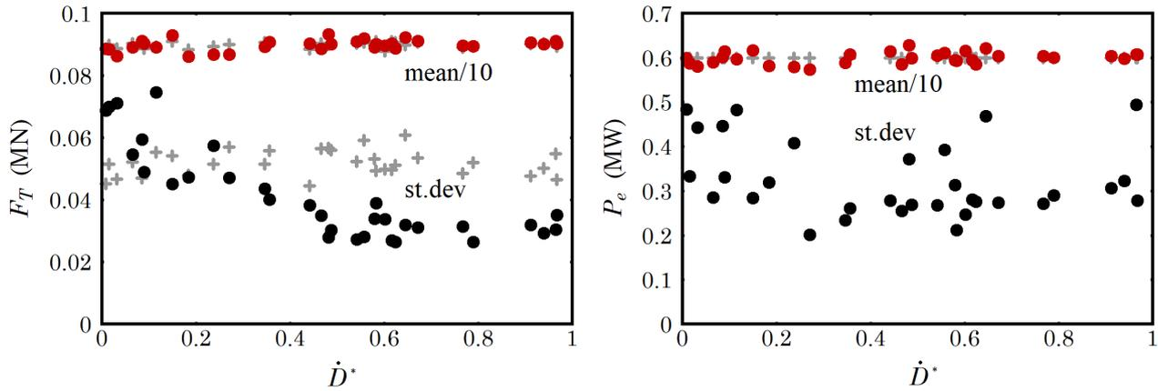
Figure 2: Trends in the mean and standard deviation of thrust and power fluctuations, as a function of damage rate. Each point represents one turbine in the TotalControl Reference Wind Power Plant. Nominal results for the case with a constant, uniform power command sent to all the turbines are shown in the background as gray points.
