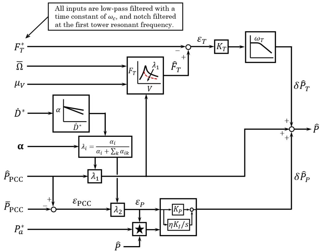
Figure 7: Architecture of the wind plant control law. The starred block provides anti-windup features; it is shown in Fig. 8.
