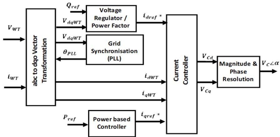
Figure 44: Block diagram of control scheme.
