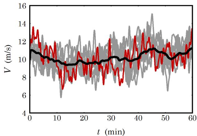
Figure 33: An example of the clustering algorithm for separating “turbulence” from “weather”, applied to simulated data with proper plant-wide correlations. The black line is the cluster wind speed, drawn from the individual turbine wind speed estimates, shown in gray. The turbine wind speed series, for which the cluster wind speed is determined, is highlighted in red.
