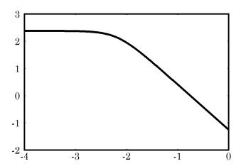
Figure 15: An example of the Von Karman spectrum,  $\mu_V = 10$  m/s, I = 0.183,  $L_u = 180$  m.
