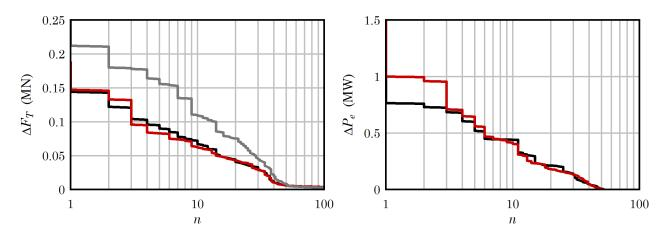
Figure 38: Rainflow-count exceedance curves of thrust and power for Turbine 1. Gray: constant power command (Scenario 1). Black: damage = 0 (Scenario 2). Red: Turbine 1 damage = 1 (Scenario 3). The gray curve is near zero in the right-hand plot. For an example of how to interpret these curves, the gray curve in the left-hand plot indicates that there are about 100 total cycles; 40 cycles that exceed an amplitude of 0.02; 10 cycles that exceed an amplitude of 0.11; and so on.
