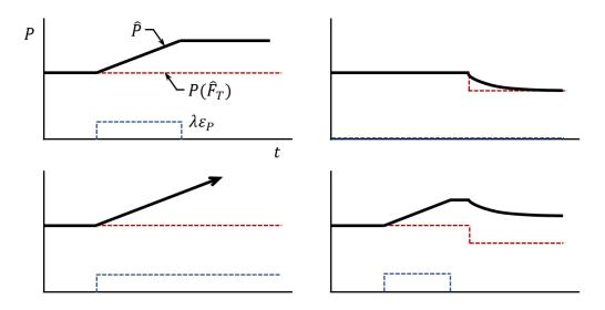
Figure 5: Sketches of the desired response characteristics of the commanded power  $\hat{P}$  under different combinations of power-tracking  $\lambda \epsilon_P$  and thrust-tracking  $P(\hat{F}_T)$  errors.
