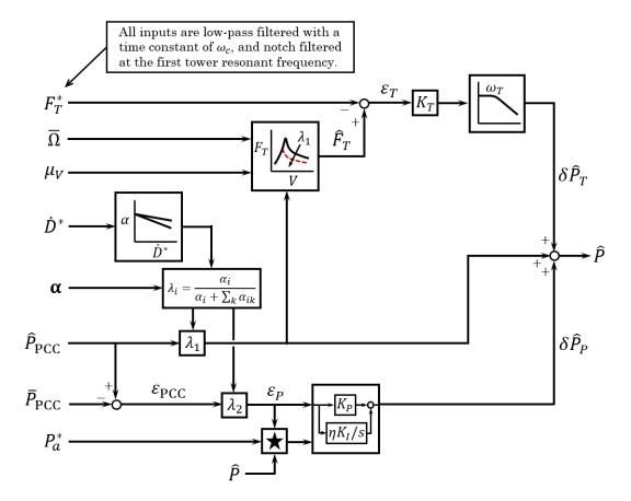
Figure 1: Architecture of the wind plant control law. The starred block provides anti-windup features.
