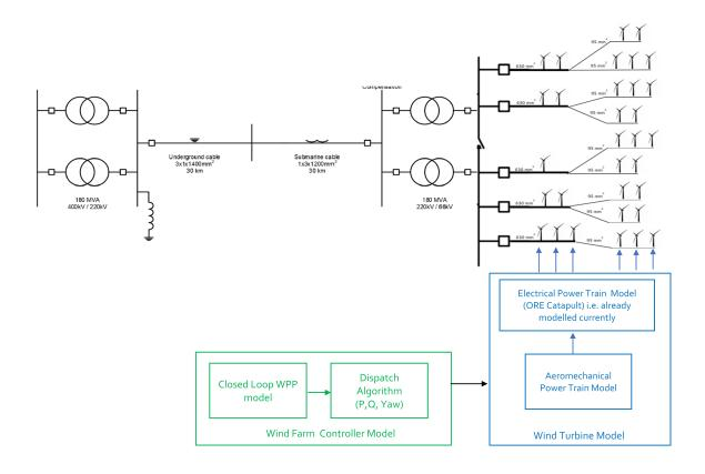
Figure 48: An illustration of representation of the hierarchical baseline PSCAD TC-RWP model.
