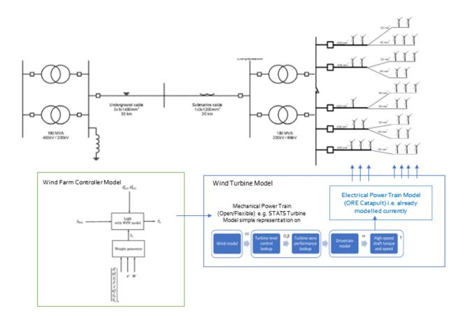
Figure 51: Block diagram of integrated WT/WPP control/PSCAD model.
