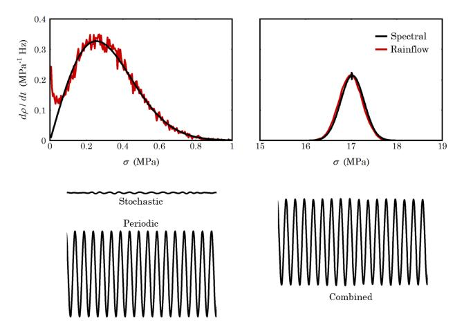
Figure 18: Cycle count density rates and samples of time series, at a location dominated by edgewise bending.
