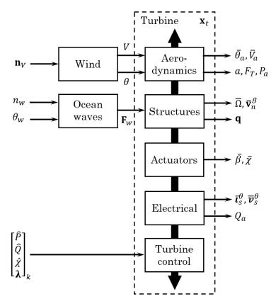
Figure 11: The architecture of the wind turbine model around which the state observer is built. The arrow behind the turbine subsystem blocks is to indicate that many internal variables, not resolved in the figure, are passed back and forth between these blocks.
