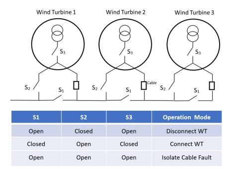
Figure 42: Wind turbine string switch gear arrangement representation in PSCAD.
