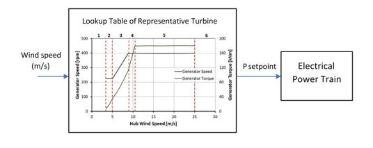
Figure 47: An example of option 2 with lookup tables of wind turbine speed and power curves.
