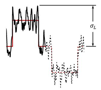
Figure 22: A high-frequency process superposed with the three-level square wave, showing the amplitude  $\sigma_L$  of the low-frequency rainflow half-cycle.
