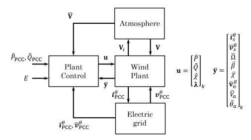
Figure 3: A high-level block diagram of a wind power plant and its surroundings, showing the interface variables.
