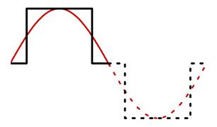
Figure 21: A cycle approximated as a three-level square wave.
