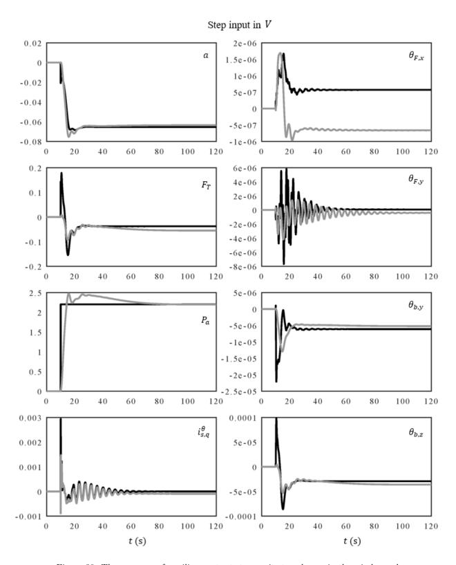
Figure 30: The response of auxiliary outputs to a unit step change in the wind speed.
