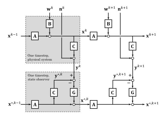
Figure 12: The discrete-time Kalman filter "unrolled" in time, as a network.
