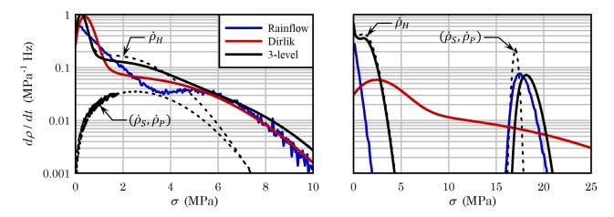
Figure 23: Combined  $(n_S, n_P, n_H)$  cycles, expressed as density rate curves. Counts obtained by the rainflow method are compared with those from Dirlik's equation and the proposed three-level method. The plot at left shows a point dominated by flapwise moments, while at the right is a point dominated by edgewise moments.
