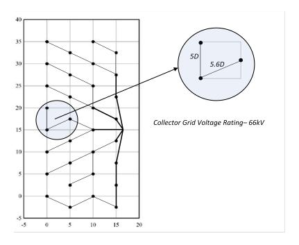
Figure 40: Collector grid cable section layout of the TC-RWP.
