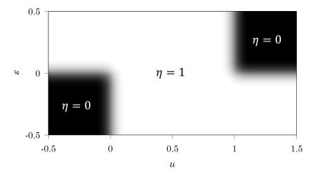
Figure 9: Output of the anti-windup block for a case in which the valid range of u is between 0 and 1. The smoothed transition between  $\eta = 0$  and  $\eta = 1$  is convenient for numerical solution of the nonlinear state equations.
