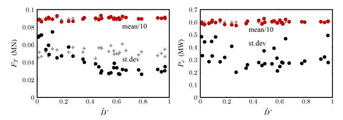
Figure 2: Trends in the mean and standard deviation of thrust and power fluctuations, as a function of damage rate. Each point represents one turbine in the TotalControl Reference Wind Power Plant. Nominal results for the case with a constant, uniform power command sent to all the turbines are shown in the background as gray points.
