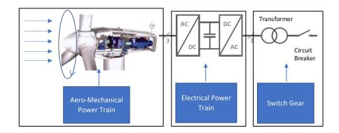
Figure 41: High level description of the Wind Turbine Model in PSCAD.
