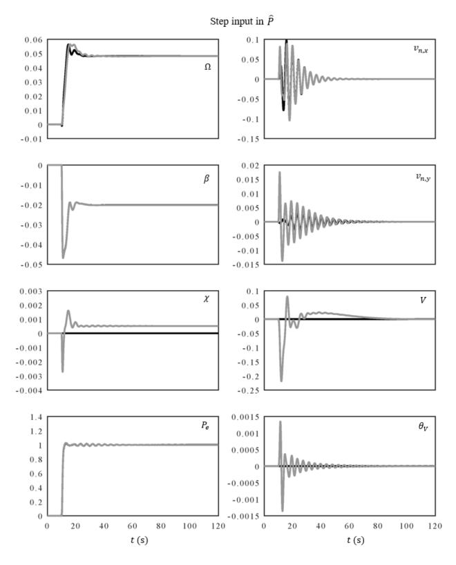
Figure 27: The response of sensor outputs to a unit step change in the electric power command. Dark lines: turbine model. Light lines: observed quantities.  $\Omega$ : rotor speed (rad/s),  $\beta$ : blade pitch (rad),  $\chi$ : nacelle yaw angle (rad),  $P_e$ : electric power (MW),  $v_{n,x}$ : nacelle fore-aft velocity (m/s),  $v_{n,y}$ : nacelle side-to-side velocity (m/s), V: wind speed (m/s),  $\theta_V$ : wind direction (rad).
