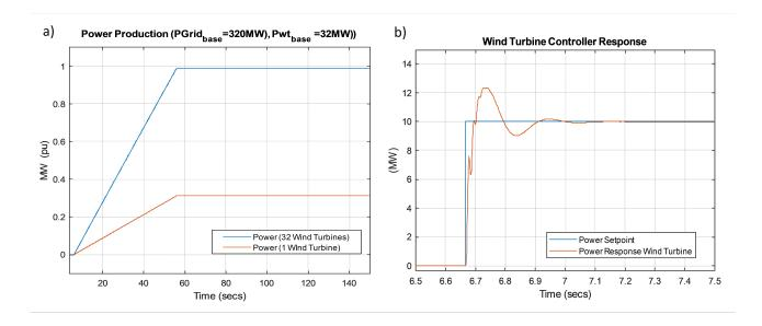
Figure 49: Simulation Results: (a) Power production with the wind turbines, (b) wind turbine controller electrical power response.
