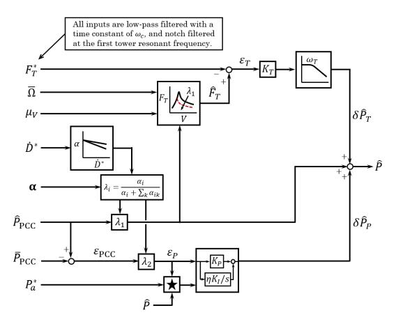
Figure 7: Architecture of the wind plant control law. The starred block provides anti-windup features; it is shown in Fig. 8.
