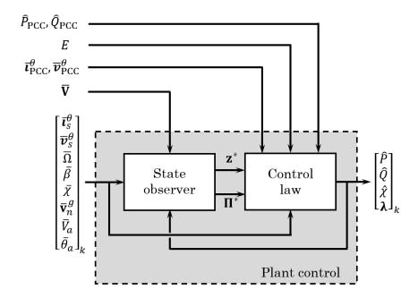
Figure 6: An expansion of the plant control block, showing how the interface variables feed into the state observer and control law.
