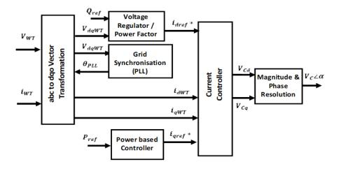
Figure 44: Block diagram of control scheme.
