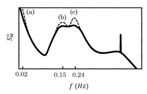
Figure 4: Active load control, illustrated on a spectrum of tower bending moments. The dashed lines indicate the original spectrum, with no active load control. (a): rejection of low-frequency aerodynamic loads. (b): rejection of wave loads. (c): active damping of resonance.
