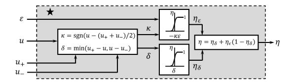
Figure 8: The block providing anti-windup features.
