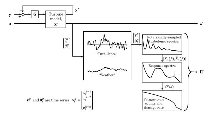
Figure 10: The architecture of the state observer, showing the embedded wind turbine model, a module that distinguishes local turbulence from broader weather patterns, and an analytical spectral model that estimates the severity of loading and fatigue.
