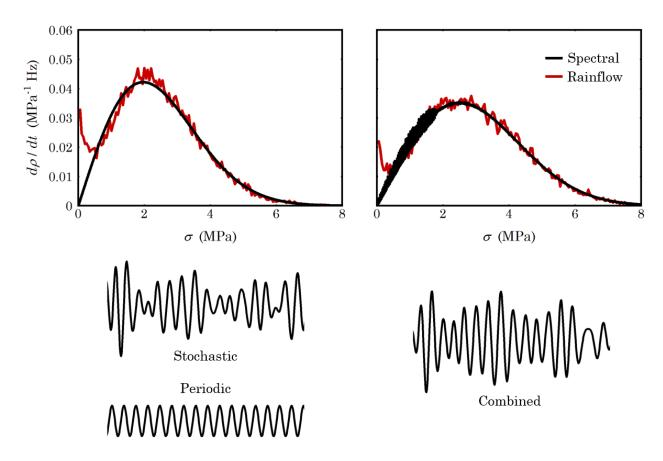
Figure 17: Cycle count density rate curves from the stochastic and periodic blade root stress spectra near the 1P frequency, along with samples of the corresponding time series. Stresses at this location are dominated by flapwise bending.
