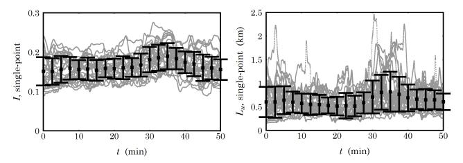
Figure 36: Single-point turbulence intensity and length scale for each turbine, derived from the turbulence cascade after a 10-minute burn-in period. The error bars indicate the standard deviation.
