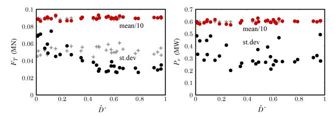
Figure 39: Trends in the mean and standard deviation of thrust and power fluctuations, as a function of damage rate (Scenario 4). Nominal results for the case with a constant power command (Scenario 1) are shown in the background.
