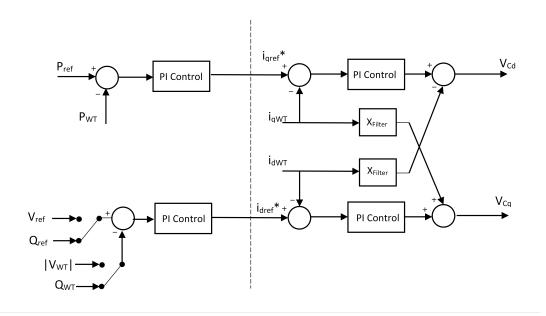
Figure 45: Control loops of Grid Side Converter.
