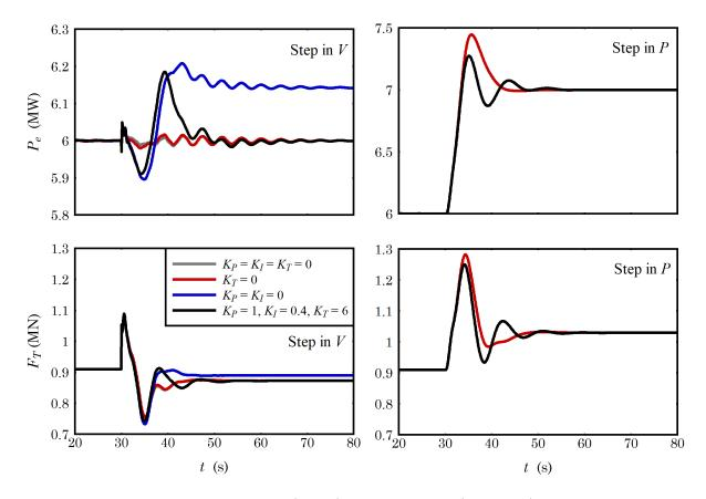
Figure 32: The response of electrical power (at top) and rotor thrust (at bottom) to unit step inputs in wind speed (at left) and power command (at right), with different gains.
