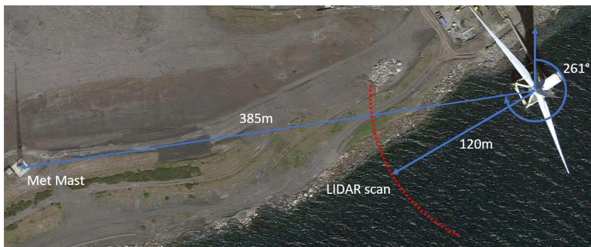
Figure 2 - Distance and orientation of the meteorological mast, turbine, and spinner LiDAR
