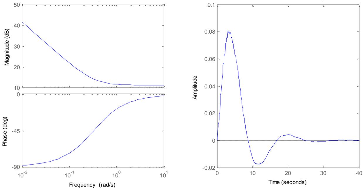
**Figure 2: (Left) Bode plot of the torque-speed PI stabilising loop. (Right) Step response of the linear model with the stabilising loop connected, from wind speed to measured generator speed.**
