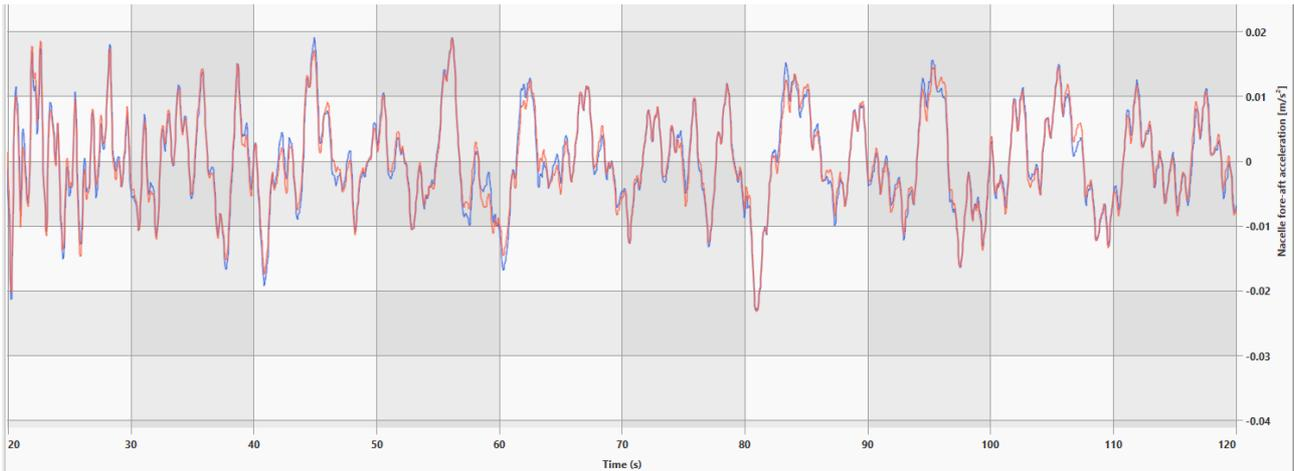
**Figure 9: Nacelle fore-aft acceleration response to steps in wind speed for base case (blue) and with higher cost on nacelle acceleration (red). The impact is very subtle but occasionally lower overshoot is evident.**
