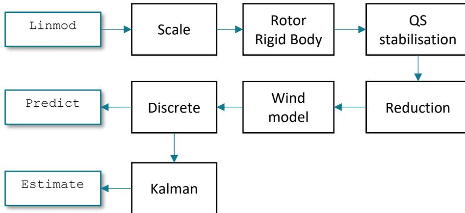
Figure 5: Adjustments made to the raw linear model to prepare it for predictions and estimation
