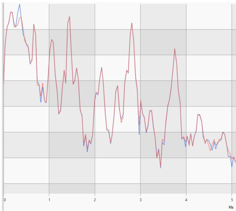
**Figure 10: Power spectral density of nacelle acceleration of the results from the test of increasing cost for that measurement. A clear reduction is seen at 0.34 Hz – the 1<sup>st</sup> tower mode. 3P falls at 0.55, where there is very little activity, suggesting the filtering works. But many other modes are visible, which are not in the prediction model and are therefore outside the capability of the cost function to reduce.**
