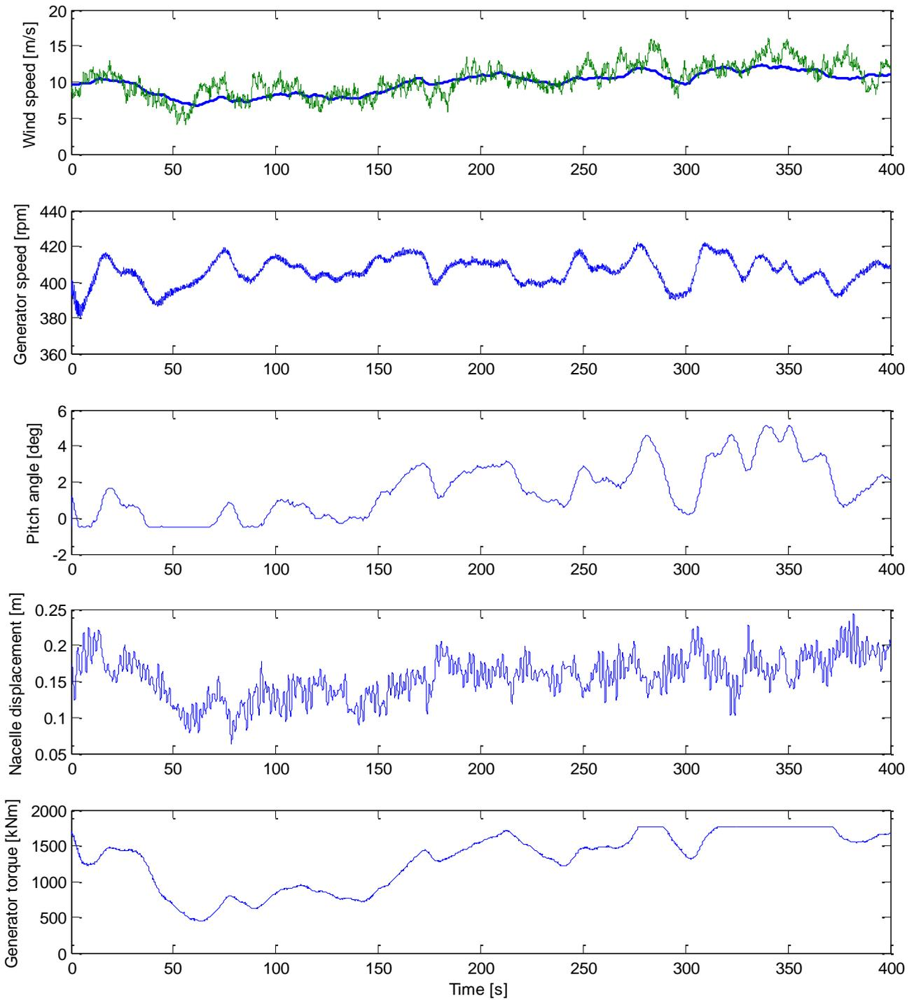
**Figure 12: Results of a 400 s turbulence case showing: rotor average wind speed (blue), hub wind speed (green), generator speed, pitch angle, nacelle displacement fore-aft and generator torque. Pitch hits constraint at 40 s; torque hits constraint at 320 s; generator speed shows tight control in high turbulence intensity.**
