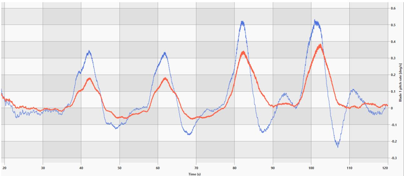
**Figure 8: Pitch rate response to steps in wind speed for base case (blue) and with higher cost on pitch rate (red). The impact is very clear, with much higher damping and much lower overshoot.**
