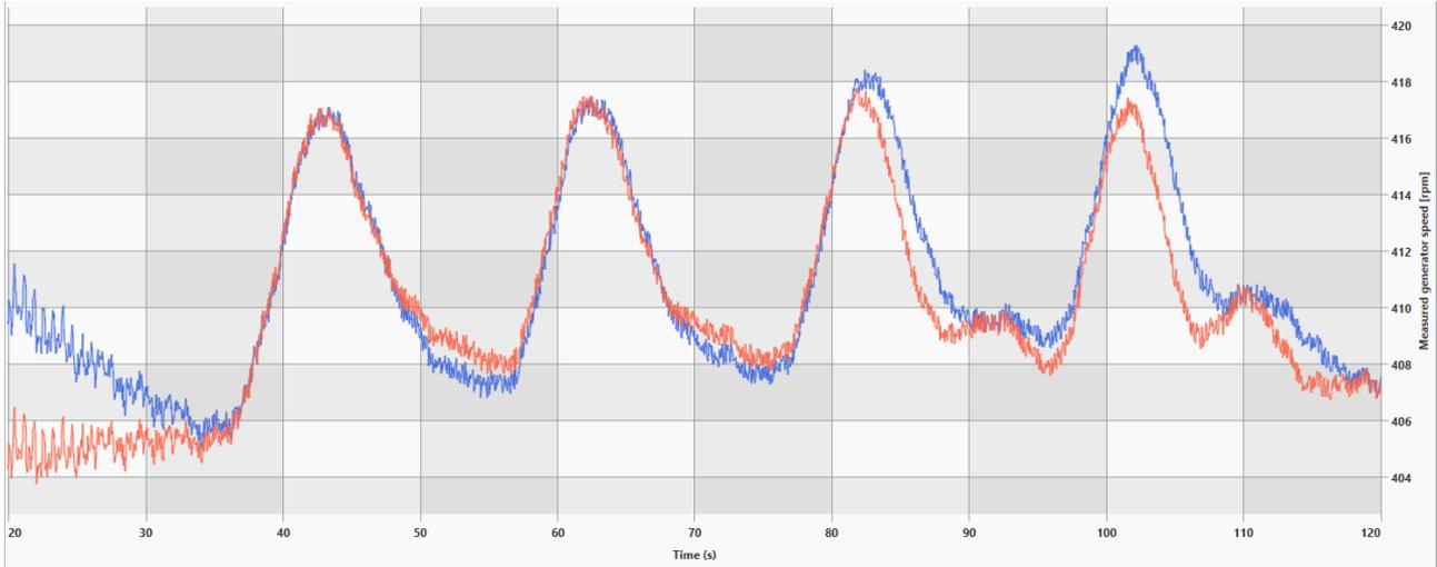
**Figure 7: Generator speed response to steps in wind speed for base case (blue) and with higher cost on generator speed (red). The initial response ( $t < 30s$ ) can be ignored due to simulation initialisation transients. Higher cost has a clear impact on tightening rotor control, e.g. 55 s and 102 s with less overshoot.**
