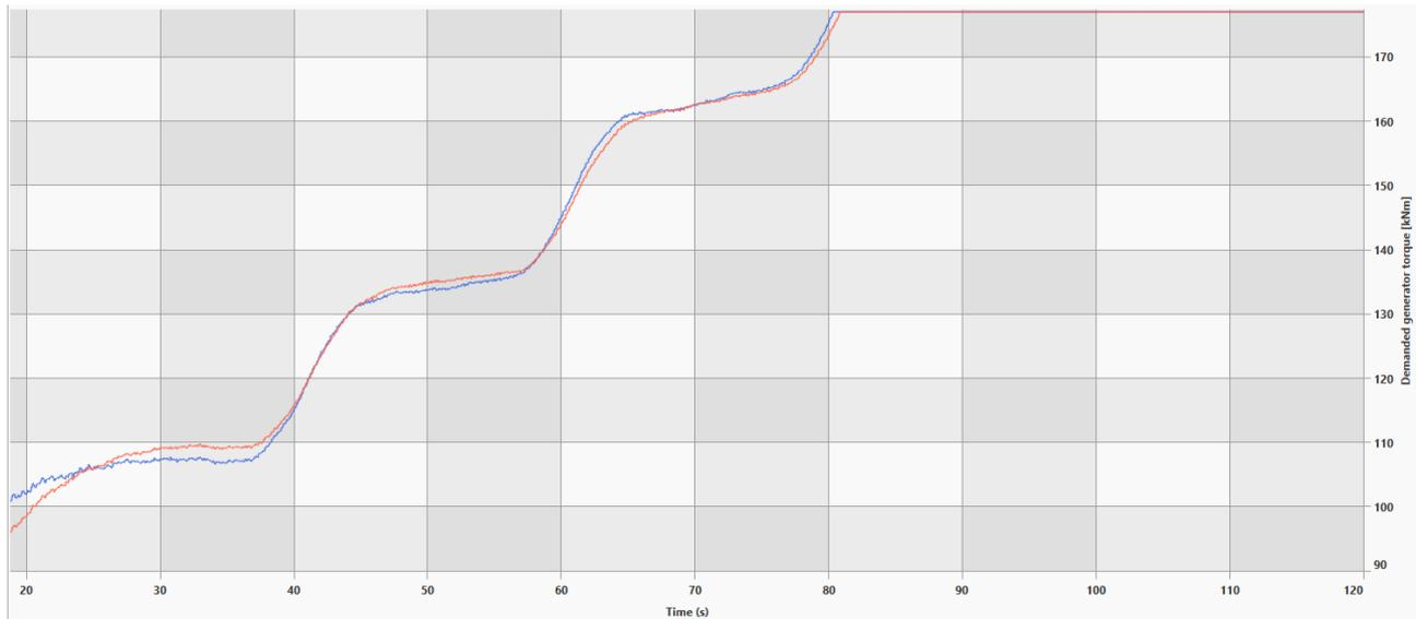
**Figure 11: Demanded generator torque response to steps in wind speed for base case (blue) and with higher cost on torque demand (red). Beyond 80 s the generator torque hits its limit but before then, there are signs that the actions are less aggressive when the cost is higher, e.g. 64 s and 78 s.**
