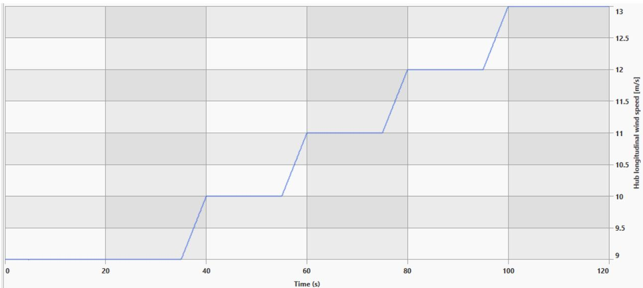
**Figure 6: Steps in wind speed from 9 m/s to 13 m/s covering control regions of variable torque and pitch angle**
