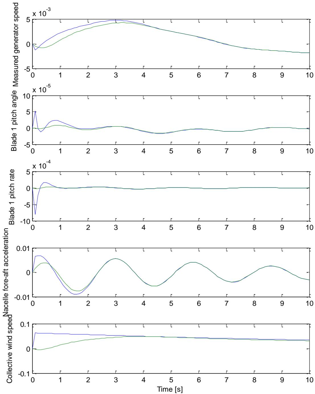
**Figure 4: The response of the full linear turbine and wind model (blue) to an impulse in wind white noise disturbance. The Kalman filter estimates the states, which are mapped back onto the measurements for comparison (green). Note the wind speed is correctly estimated after 4 s, purely from the four measured signals.**
