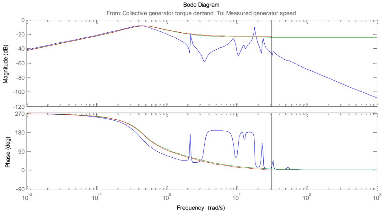
**Figure 3: Bode diagram from generator torque demand to measured generator speed for the stabilised linear model (blue), the reduced model (green) and the discrete model (red, with Nyquist limit shown as a black bar). Clearly there are many modes ignored by the reduced model, which are thereby uncontrolled.**
