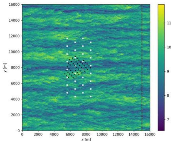
The precursor fields are large enough to contain the virtual wind farm, here either the newly defined reference wind farm (white turbine locations) or the Lillgrund wind farm (black dots) which is used for the measurement campaign.
