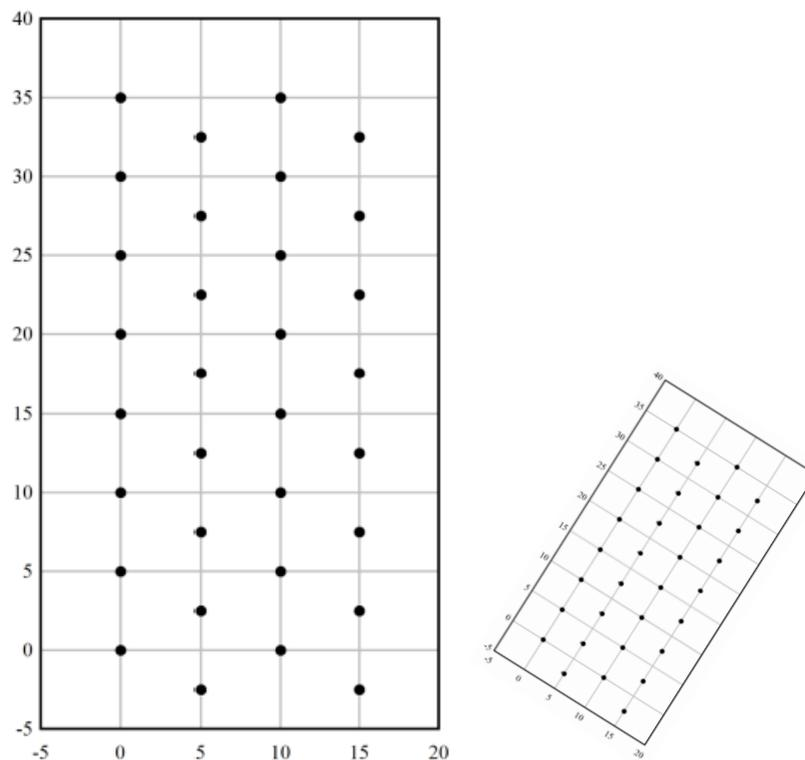
The farm layout can be rotated to have a long farm, a wide farm, and different inter-turbine distances when the wind farm is turned.
