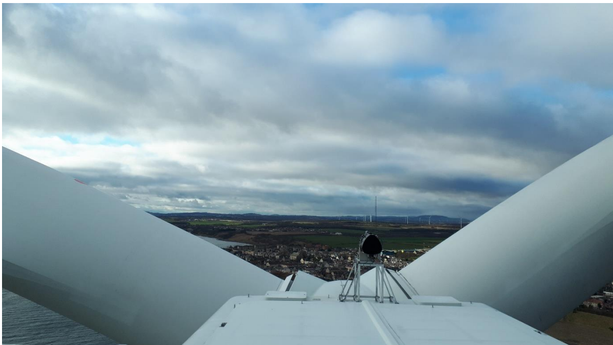
Figure 4: DTU SpinnerLidar installed on the Levenmouth turbine nacelle roof in Scotland, measuring the rotor inflow conditions.
