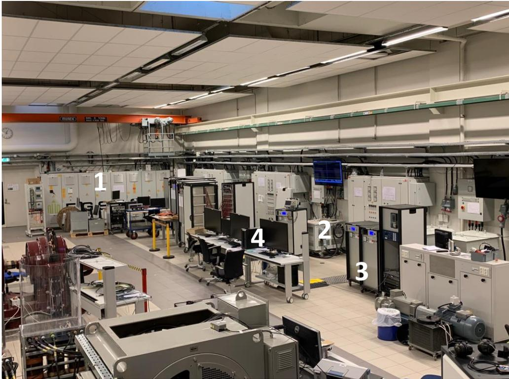
**Figure 4-3:** Norwegian National Smart Grid Laboratory. Marked in the figure: Grid emulator (1), Power electronics converters (3), Transformers (2), Control interface (4)
