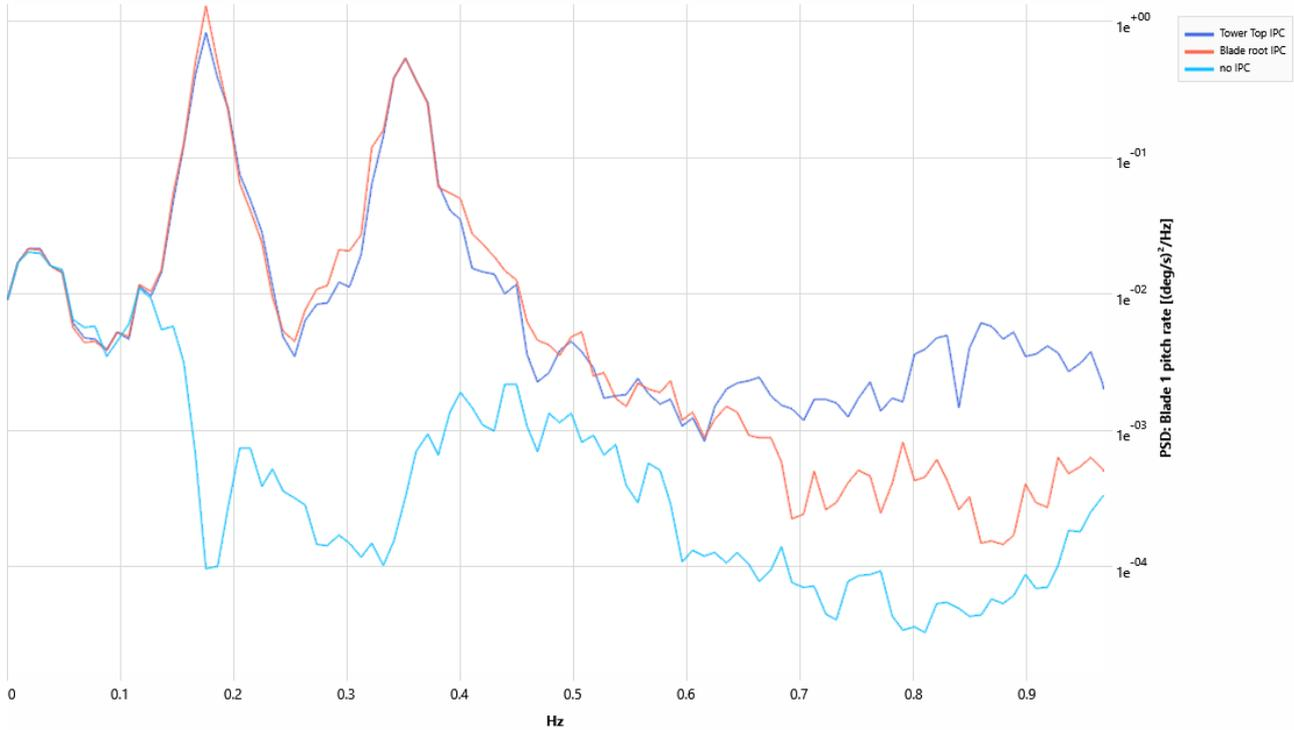
**Figure 28** Effect on Blade 1 pitch angle of 2P IPC. Blade root sensors (orange) and tower top sensors (blue)
