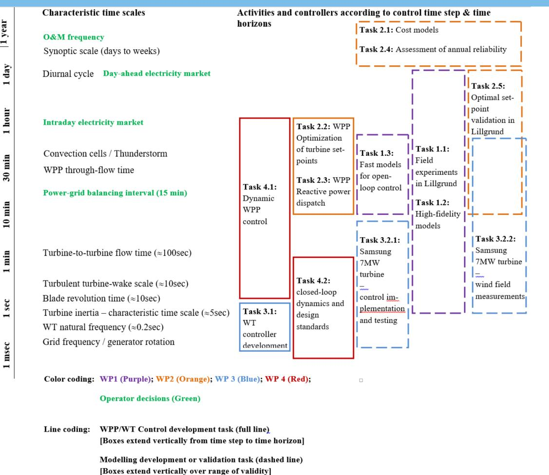
TotalControl is built on a hierarchy of controllers, each reacting at different time scales and control time steps. At the *slowest control level* the WPP is quasi-statically adapting its WT active and reactive power set points and WT yaw angles, adapting to slowly changing environmental conditions and market elements. A *second control level* is the WT controller, accepting power set points from the quasi-steady control levels.
